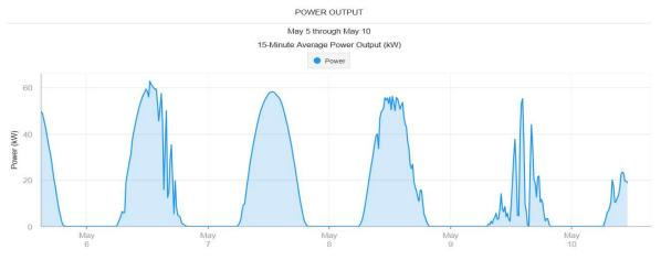
Figure 3-5 Solar Production Variation and the Need for System Regulation<sup>1</sup>
