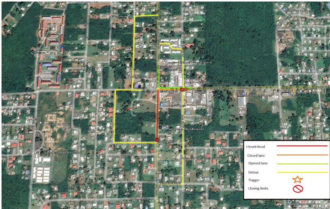
Figure 1: Highlighted red line indicates road closure, while yellow line indicates available detour route and green line represents opened lane.
