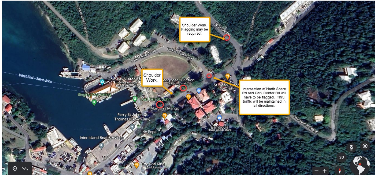
Figure 3: Highlighted red circles indicate manholes and descriptors outline shoulder work and where flaggers will be present on St. John. Thru traffic will be maintained in all directions.
